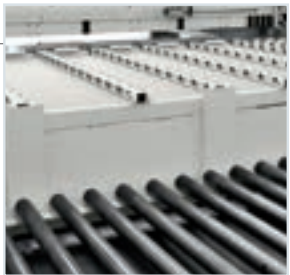
Loading platform High customisation and maximum versatility according to the user's requirements, with powered roller conveyor with trilateral loading (option on gabbiani st).
